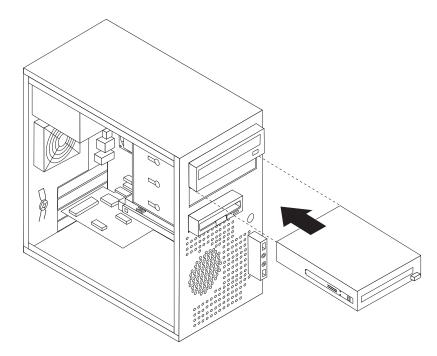
Figure 15. Installing the drive
